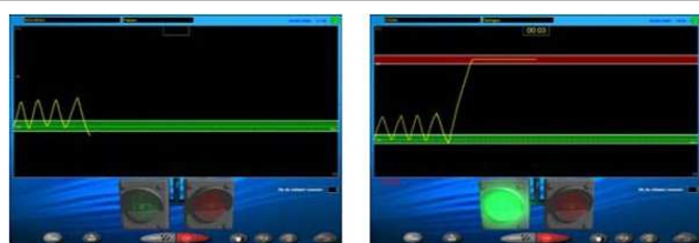
Figure 2 Screens during a fraction. After normal sinusoidal breath, the gating level is displayed in red.
