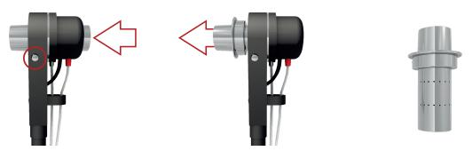
The Honey Comb Tube is an assembly of different elements (tube, security locking, central axe, sheet metal strip) all made with austenitic stainless steel.
